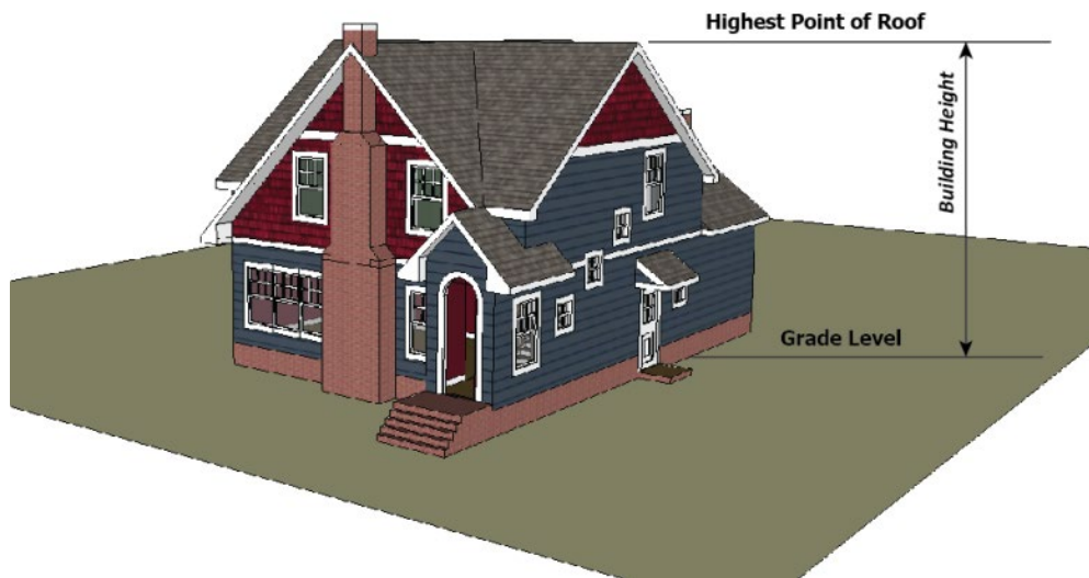
Figure 5-L: Measurement of building or structure height
