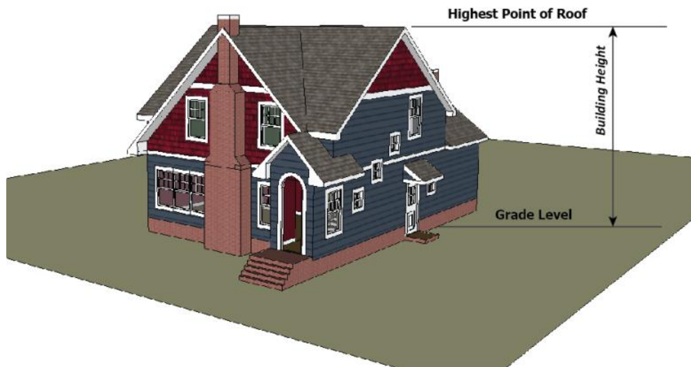
Figure 5-L: Measurement of building or structure height
