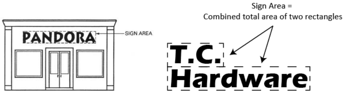
Figure 13-D: Illustration of sign area calculation for two differently shaped wall signs with individual letters.
