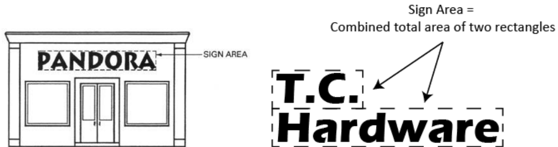
Figure 13-D: Illustration of sign area calculation for two differently shaped wall signs with individual letters.
