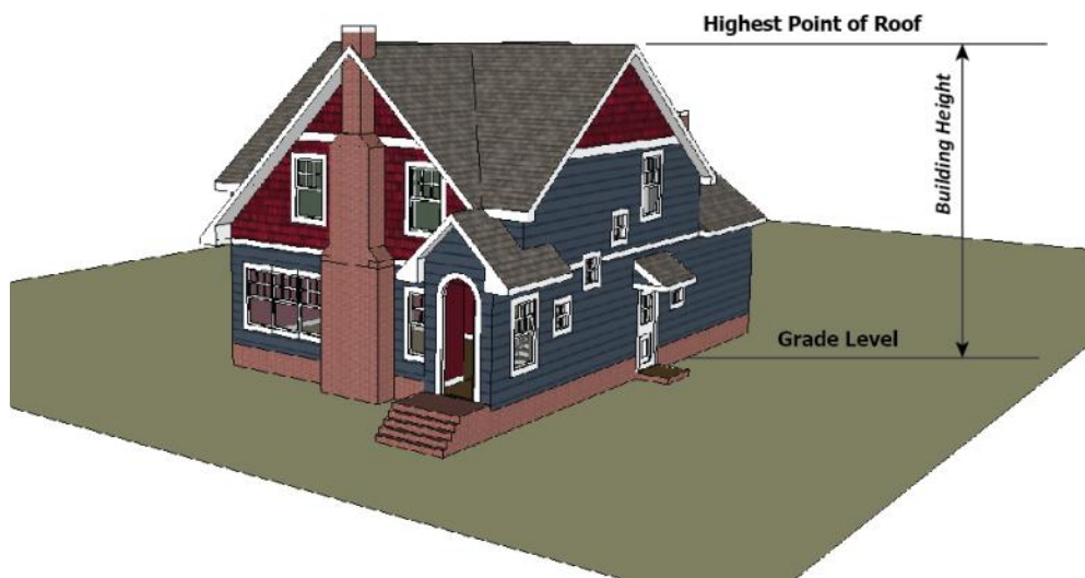
Figure 5-L: Measurement of building or structure height
